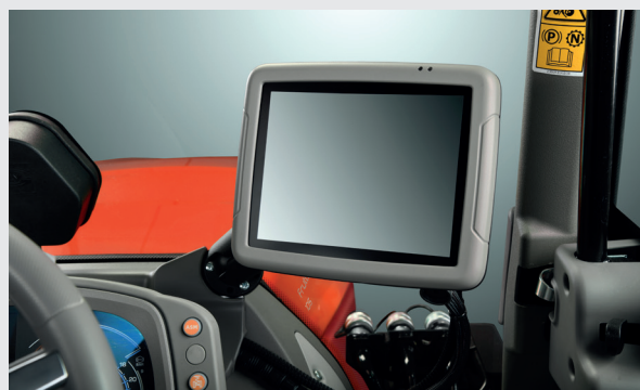
The Frutteto CVT, Frutteto CVT S and Frutteto CVT V can also be equipped with the 8" iMonitor, installed on the right hand corner of the dashboard with an adjustable mount.
